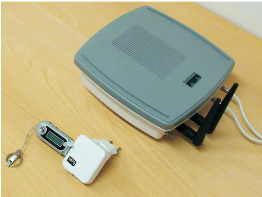
Figure 4.2: FM transmitter and Wi-Fi access point.
